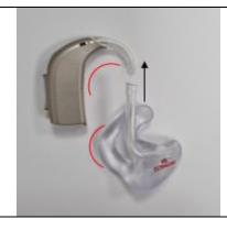
Once the tubing is cut to the right length, reattach the mould to the hearing aid.
