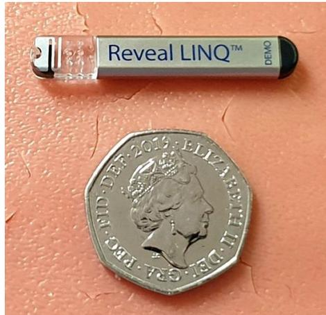
An ILR (from Medtronic) compared with a 50p coin
