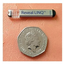
An ILR (from Medtronic) compared with a 50p coin
