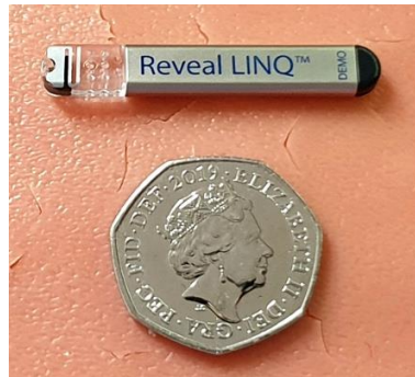
An ILR (from Medtronic) compared with a 50p coin
