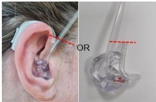
3. Once the tubing is cut to the right length, reattach the mould to the hearing aid. Ensure the curve of the ear mould matches the curve of the hearing aid, so that it sits correctly on the ear.
